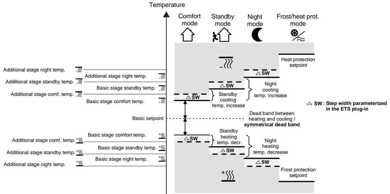
If enabled in the ETS, 6 temperature setpoints can be varied in "heating and cooling" control option. Depending on the temperature decrease, increase or dead zone parameterized in the ETS, all temperature setpoints are derived from the basic setpoint temperature.
