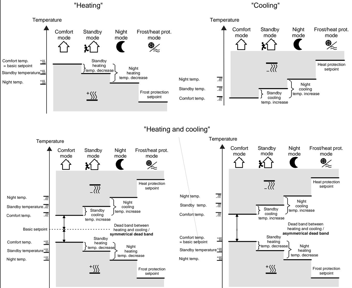
Temperature control with additional stage considering as an example "heating and cooling" with symmetrical dead zone...
