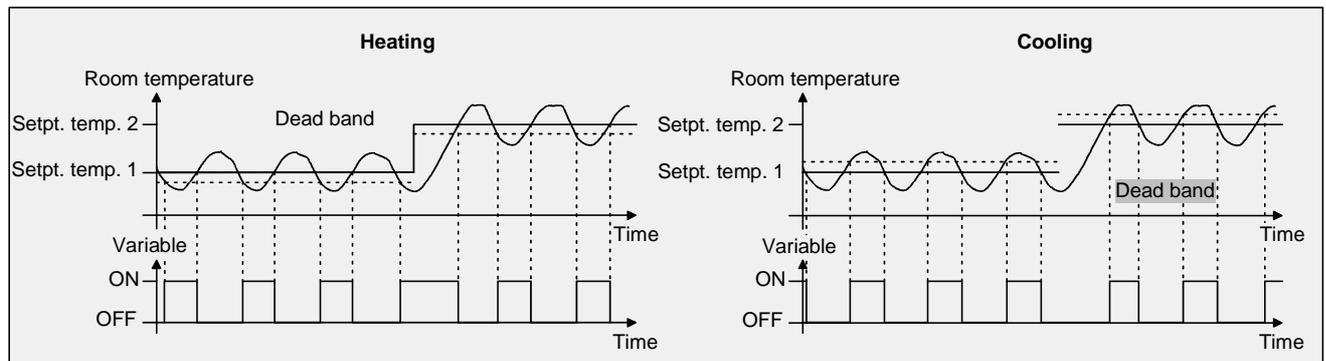
An additional 2-state control heating or cooling stage works in exactly the same way as the 2-state control of the basic stage. The difference is that the setpoint and the hysteresis values will shift by taking into account the parameterized stage offset.
