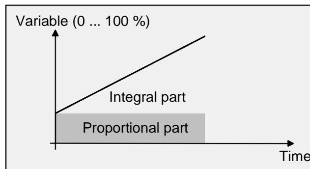
An additional PI controlled heating or cooling stage works exactly as the PI control of the basic stage. The difference is that the setpoint will shift by taking into account the parameterized stage offset.
