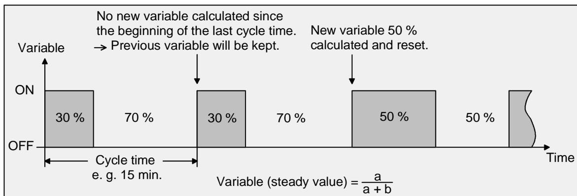
With an actuating variable of 0 % (continuously switched-off) or 100 % (continuously switched-on) an actuating variable telegram according to the actuating variable value ("0" or "1") is output after a cycle time has elapsed. With this type of control, the 'clipping' behaviour (cf. "continuous PI control") is active as well.
