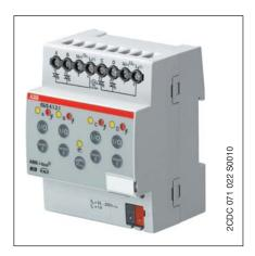
The Electronic Switch Actuator ES/S 4.1.2.1 is a modular installation device in Pro M design. The device features four semiconductor outputs for control of electrothermal valve drive in heating and cooling systems. The outputs can be operated with either DC or AC voltage (24...230 V AC/DC). Each output is short-circuit and overload protected. The outputs can be directly controlled using the manual pushbuttons. The LEDs on the front of the device signal the status of the outputs.
