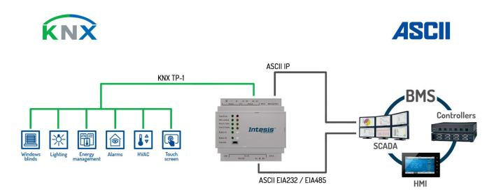
Figure 1.1 Integration of KNX into ASCII IP or ASCII Serial control and monitring systems
