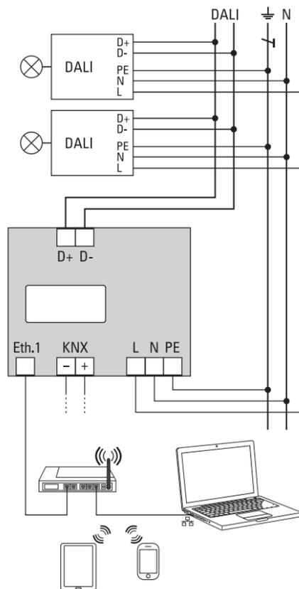
After all the connections have been completed and the power supply is turned on, the product name and firm ware version appear on the display. You can now start the commissioning of the DALI line and programming with ETS.
