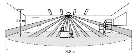
When a person is walking, a larger area of detection is available. The reference level for detection is the floor. Also the position of the KNX ARGUS Presence in relation to the moving direction influences the detection.
