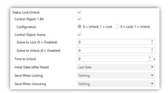
Figure 11. Enabling the channel by using a 1-bit object
