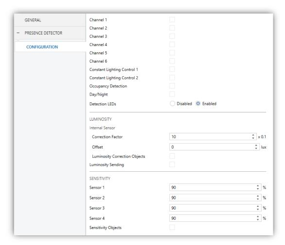
Figure 4. Presence detector. Configuration
