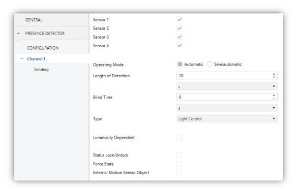
Figure 8. Configuring a presence detection channel
