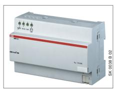
The Battery Module is a sealed lead acid battery which acts as a back-up energy source for the ABB i-bus<sup>®</sup> EIB system voltage during mains failures. The Battery Module can only be used in combination with the Uninterruptible EIB Power Supply SU/S 30.640.1. The Battery Module is a DIN rail mounted device and can simply be snapped onto the mounting rail under the SU/S 30.640.1 in the distribution board.
