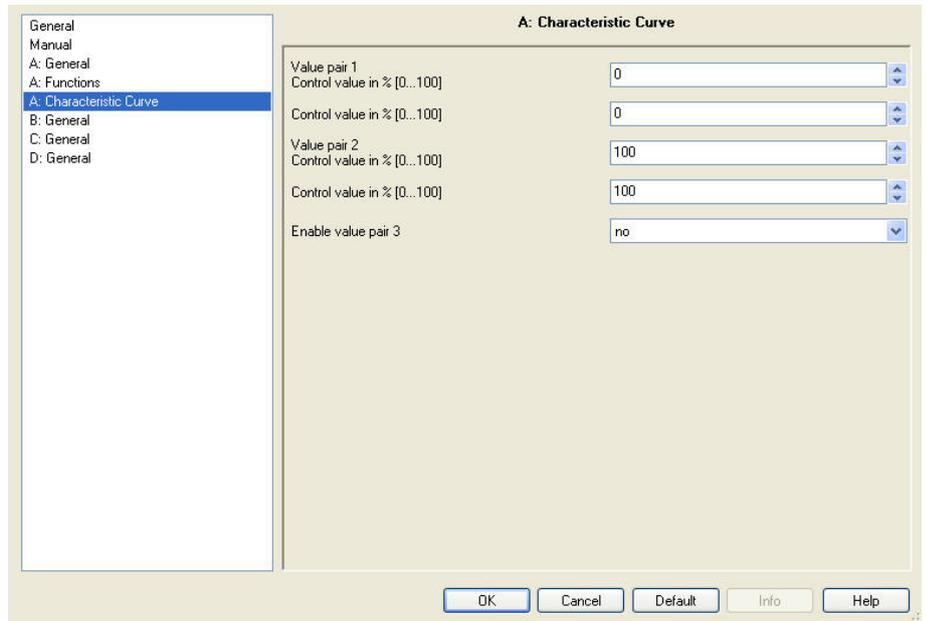
In this parameter window, an adaptation of the valve drive to the valve that is employed can be undertaken using the characteristic curve correction. A characteristic correction optimizes the control behaviour of the system if required.
