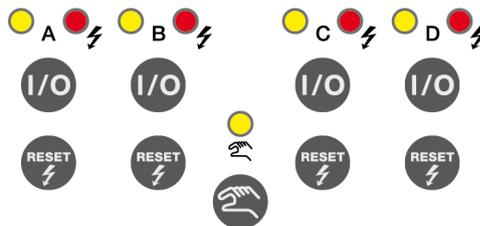
Accordingly, the wiring of the loads connected to the outputs can be verified during commissioning. You can, for example, ensure that the connected valve drives open or close the valves correctly. If bus voltage is not yet available at the time of commissioning, the device can be supplied with power for manual operation using the Power Supply NTI/Z.
