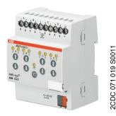
The 4-fold Blind/Roller Shutter Actuator is used to automatically control independent 24 V DC drives, for positioning blinds, roller shutters, awnings and other shading products via ABB i-bus<sup>®</sup> KNX. The devices are also used, for example, to control doors, windows and ventilation flaps. The travel times of the drives are automatically determined via end position detection and stored.
