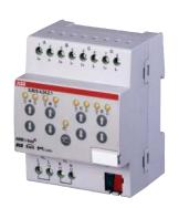
The SMI LoVo Blind/Shutter Actuator SJR/S 4.24.2.1 controls four independent groups each with up to 4 SMI LoVo blind or shutter drives (24 V) for positioning blinds, shutters, awnings and other shutters/blinds via ABB i-bus® KNX.
