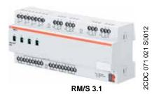
The Room Master is a modular installation device (MDRC) in Pro  $\it M$ design. It is intended for installation in the distribution board on 35 mm mounting rails. The assignment of the physical addresses as well as the parameterization is carried out with the ETS and the current application program. The RM/S is powered via the ABB ibus® and does not require and additional auxiliary voltage supply. The device is ready for operation after connecting the bus voltage.
