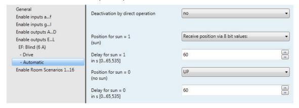
The Automatic function enables a simple automatic sun protection and automatic protection against dazzle in conjunction with the JSB/S.
