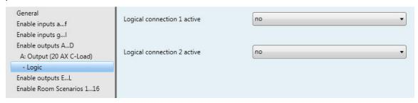
The function Function Logic provides up to two logic objects for each output, which can be logically linked with the communication object Switch.
