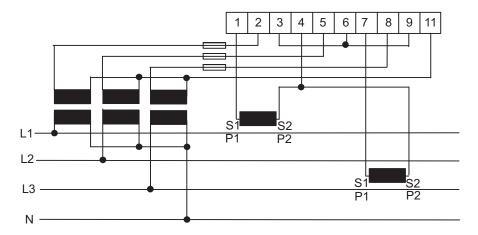
The following diagram shows a 3-element transformer connected meter with 2 current transformers and a floating neutral:
