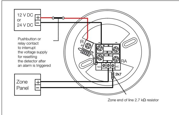
Variant 2: With monitoring of the supply voltage and detector removal
