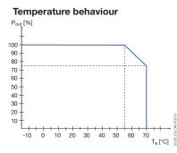
Characteristic curve of temperature at Uout
