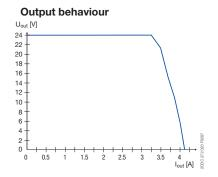
Characteristic curve of output at  $T_a = 25 \ ^{\circ}C$
