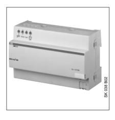
The Battery Module is a sealed lead acid battery which acts as a back-up energy source for the EIB system voltage during mains failures. The Battery Module can only be used in combination with the Uninterruptible EIB Power Supply. The Battery Module is a DIN rail mounted device and can simply be snapped onto the mounting rail under the Uninterruptible EIB Power Supply in the distribution board.
