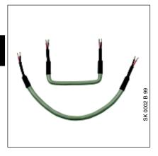
The wiring jumpers VB/K 270.1, VB/K 200.1 and VB/K 100.1 are used to connect devices to the EIB that have a bus connecting terminal at the front of the device. They are suitable for wiring in the distribution board as well as in the control cabinet on a longer mounting rail. There are no limitations regarding length as there are for the data rail and a connector is not required.
