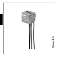
EIB devices are protected internally against overvoltage impulses up to 2 kV (1.2/50). The overvoltage protector is used to protect them beyond this level. It takes the form of a one-part blue bus terminal with three fixed core wires.
