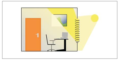
Fig. 6: Daylight redirection
