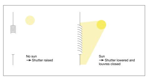
Fig. 5: Method of functioning of automatic sun protection
