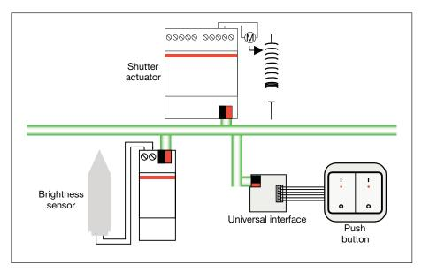
Fig. 8: Planning a simple automatic sun protection system
