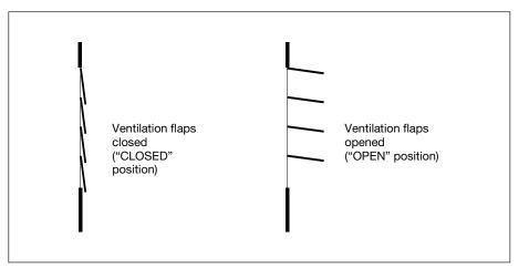
Fig. 11: Open/close ventilation flaps
