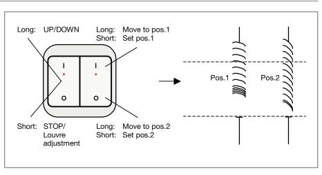
Fig. 4: Move to preset position and store preset position
