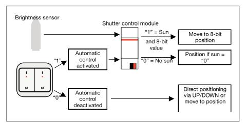
Fig. 9: Structure of an automatic sun protection system which tracks the position of the sun
