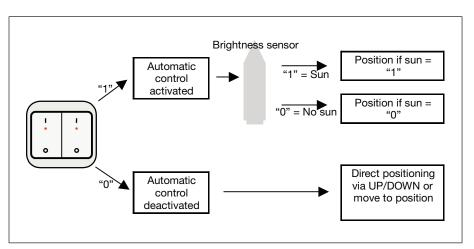
Fig. 7: Structure of a simple automatic sun protection system
