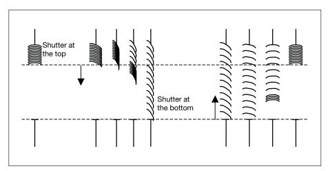
Fig. 2: Louvre position when raising and lowering the shutter
