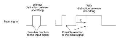
Diagram 1: Distinction between short/long operation in the "Switch sensor" function
