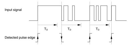
When a pulse edge is detected at the input, further pulse edges are ignored for the duration of the debounce time  $T_D$ .
