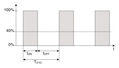
During  $t_{ON}$ , the value is triggered with OPEN ("ON phase"). During  $t_{OFF}$ , the value is triggered with CLOSE ("OFF phase"). Due to tON = 0.4 x T<sub>CYC</sub>, the value is set at approx. 40%. T<sub>CYC</sub> is the so-called PWM cycle time for continuous control.
