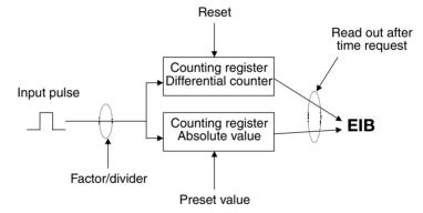
Apart from the absolute counter, it is possible to enable a differential counter which measures differential values (e.g. comparable with a daily mileage indicator). To be able to adapt the count rate, factors and dividers can be set for both counters.
