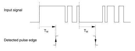
Since only two pulse edges remain stable for the duration of the minimum operation time  $T_{\mbox{\scriptsize M}},$  only these edges are recognised as valid.
