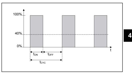
Bottom right graphic: Control of electronic relay (heating actuator)
