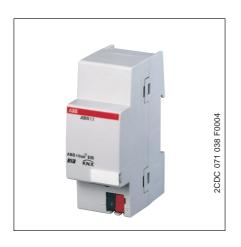
The shutter control unit controls shutter actuators with the functions of anti-glare protection and daylight redirection via the ABB i-bus® EIB. The current position of the sun is always calculated and logically combined with a threshold value for the sun's intensity so that the shutter is only moved into the calculated position when the sun is actually shining.
