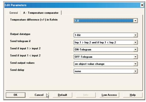
Diagram 6.2.7.1: 'A - Temperature comparator' in the default setting
