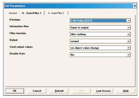
Diagram 5.2.8.1: 'A - Gate/Filter 1' in the default setting
