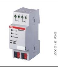
The diagnosis and protection module enables quick diagnostics of the bus state and indicates telegram traffic via an LED. A bus fault (U<U\_min) is indicated by normally open and normally closed contacts. The DSM incorporates a suppressor diode which suppresses transient overvoltages and interference voltage spikes on the EIB.
