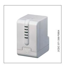
The Electromotor Valve Drive ST/K 1.1 is a proportional valve drive for controlling heating valves via the ABB i-bus® EIB. The valve drive is mounted on thermostat valve bases. The control is carried out via a continuous EIB / KNX room thermostat.
