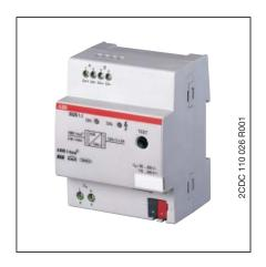
The 1-fold EIB / DALI Gateway DG/S 1.1 is a modular installation device in proM design (4 MW) for installation in the distribution board on 35 mm mounting rails. The DALI gateway can integrate devices with DALI interfaces into an EIB / KNX building installation.
