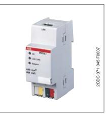
The IP Router 2.1 is a modular installation device (MDRC) and forms the interface between KNX installations and IP networks. It can be used as a fast line and area coupler and can utilise the local network (LAN) for fast exchange of telegrams between the lines/areas.
