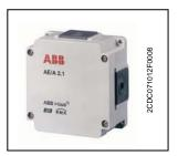
Analogue Input AE/A 2.1 is used to record analogue data. Two conventional sensors can be connected to AE/A 2.1. The connection to the bus is established using a pluggable screw terminal. The device is ready for operation after connecting the bus voltage. No additional auxiliary voltage is required.
