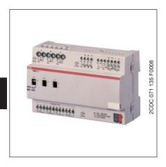
The Room Master Basic is a modular installation device (MDRC) in ProM design. It is intended for installation in the distribution board on 35 mm mounting rails. The assignment of the physical address as well as the parameter settings is carried out with ETS 2 from version V1.3a or higher.
