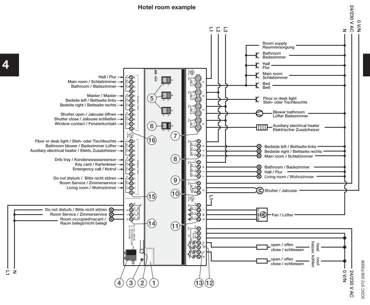
RM/S 2.1 with electro-thermal valve drives
