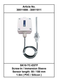
Sensor: PT1000 Screw-In / Immersion Sleeve V4A, Ø 9mm max. pressure 40 bar Connecting Cable: 15m PVC 1.5m Silicon -35 .. +105°C Measurement Range: -50 .. +180°C Silicon Resolution: 0.02°C Accuracy Class B, ±(0.3°C+0.005\*T) Operating Temperature: -25 .. +80°C Storage Temperature: -25 .. +80°C Protection Class: IP54/65
