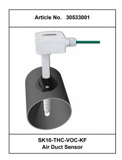
Duct diameter inside: min. 150mm Measurement Range Temperature: -25 .. +80°C Resolution: 0,02°C  $\pm 0.4$ °C (5..60°C), else  $\pm 0.8$ °C Accuracy: rel. Humidity: 10 .. 95% r.H Resolution: 0.02% r.H Genauigkeit: ± 3% r.H (20..80%) @ 25°C, else ± 5% 400 .. 10000 ppm VOC level: CO2 equivalents -25 .. +80°C Operation Temperature: Storage Temperature: -25 .. +80°C Protection Class: IP54/65
