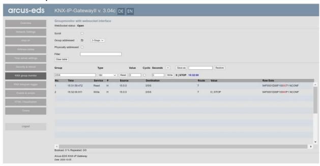
With the KNX group monitor it is possible to monitor or send telegrams on the KNX bus in real time. The side of the KNX group monitor is divided into a configuration area and a telegram area.
