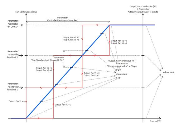
This is used as an input for the calculation of the "Output, Fan VX" 1-bit objects, with the internal steady value of the object "Output, Fan Continuous [%]" as reference value. This is formed according to the error ( Setpoint - Temperature ) and in dependency of the parameter "Controller Fan Proportional Part ( Controller Page Fan ), Page 121". The formula for the steady value is {Error \* ( 100% / parameter "Controller Fan Proportional Part" )}.
