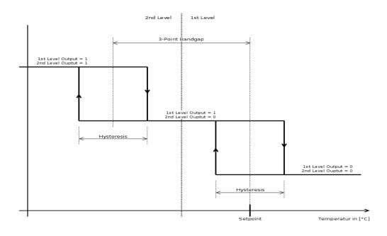
The figure shows a simple 3-point-controller heating. The setpoint in the 1st level is at half the hysteresis value. The hysteresis for both levels is the same and set by the parameter "Hysteresis" (Temp. Controller Heating / Cooling ). The gap between the two levels is set by the 3-point bandgap. For cooling mode, the figure can be viewed mirror-inverted at the setpoint.
