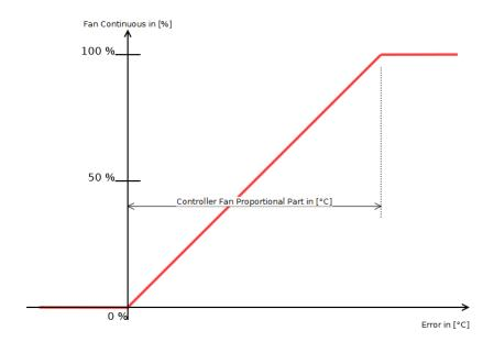
Fan Continuous = Controller Fan Proportional Part · (setpoint – Temperature)
