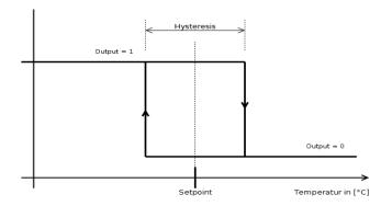
The figure shows a 2-point-controller heating. The hysteresis is set by the parameter "Hysteresis" (Temp. Controller Heating / Cooling ) and the setpoint is at half the hysteresis value. For cooling mode, the figure can be viewed mirror-inverted at the setpoint.
