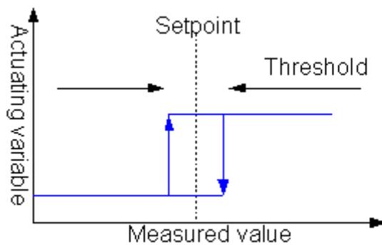
**Two-Position Control with Pulsed Output:**
