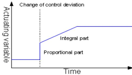
**Continuous PI Control with Pulsed Output (PWM):**
