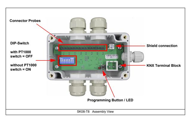
The temperature sensors of the SK08-T8 are connected in series. Therefore, any unused input must be short-circuited with the DIP switch. The channel is short-circuited and deactivated when the associated DIP switch is set to "ON" or "1".
