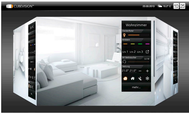
Home screen of the CUBEVISION with Instant Control Panel (ICP)
