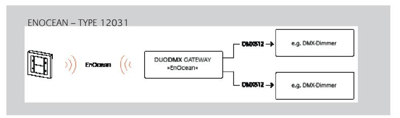
The DUO**DMX** GATEWAY 12031 receives the control command via the built-in EnOcean module. The EnOcean signals are converted into DMX packets and forwarded to the DMX dimmers.
