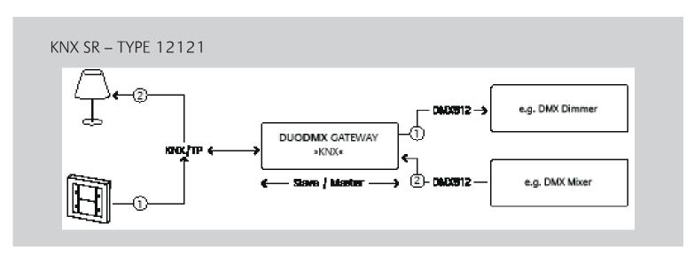
① The DUODMX GATEWAY 12121 SR is connected to the KNX bus and receives its control commands directly via the KNX bus. The DMX packages for the DMX dimmers are then triggered. ② The DMX mixer (DMX Master) is connected to the DUODMX GATEWAY (DMX Slave). The DMX packets are converted into KNX telegrams and sent to the KNX devices.
