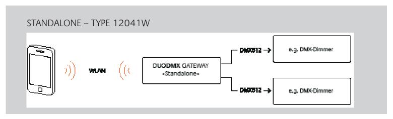
The smartphone and the DUO**DMX** GATEWAY 12041W with integrated WLAN module communicate over the network. The smartphone application sends control commands to the gateway via WLAN. These are forwarded by the DUO**DMX** GATEWAY to the DMX dimmers.
