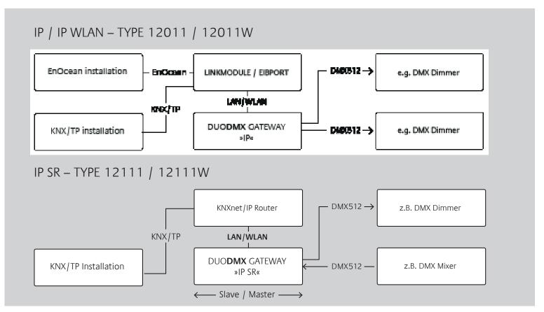
**IP variant:** As an IP variant, the DUO**DMX** GATEWAY 12011 receives the commands via KNXnet/IP routing. The DMX packets are then forwarded to the DMX world.
