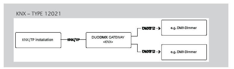
The DUO**DMX** GATEWAY 12021 is connected to the KNX bus via twisted pair. It receives its control commands directly via the KNX bus and forwards DMX packets to the DMX dimmers.
