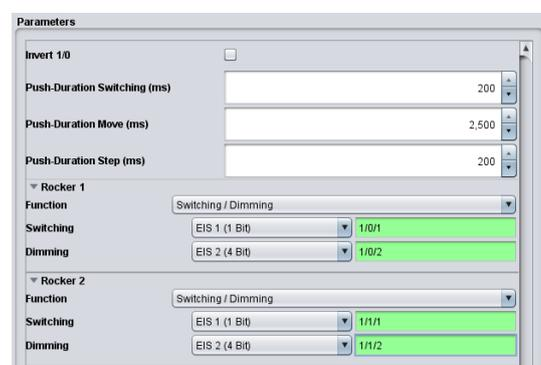
Figure 42: Receiving KNX parameters
