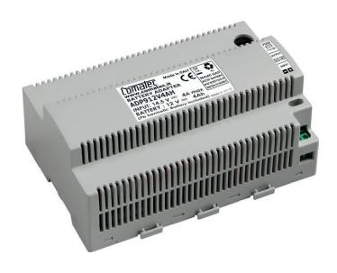
With the »ADP9« accumulator, you can realise a cost-effective emergency power supply in connection with our 12 V power supply unit for example for the EIBPORT. In the event of a power failure or a voltage interruption, the power supply is ensured for at least 6 hours (at a load of 5 W). The battery is designed for tophat rail mounting and has an integrated fuse to protect the battery.
