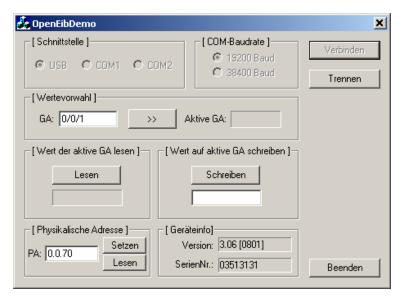
In the example the EIBWeiche has the physical address "0.0.70". If you want to change this address, you have to enter the new address and click on the button "Setzen".
