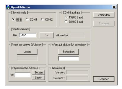
Now just select the interface (USB, COM1/2), and click on the button "Verbinden". So the area beneath is filled with the device infos (firmwareversion, serial number) and the actual phys. address:
