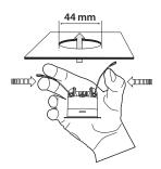
The detector has been designed and developed specifically for installation in suspended ceilings. A circular opening of diameter 44 mm must be produced in the ceiling.
