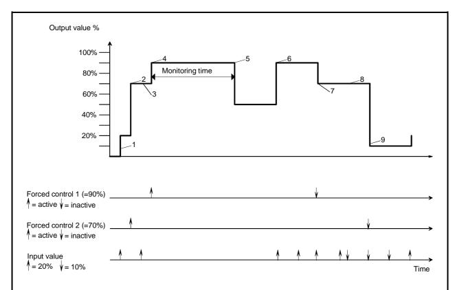
The diagram above shows the interaction of the communication objects "Input value" and "Forced guidance" in conjunction with a monitoring cycle. The arrows indicate the time when a telegram is transmitted.
