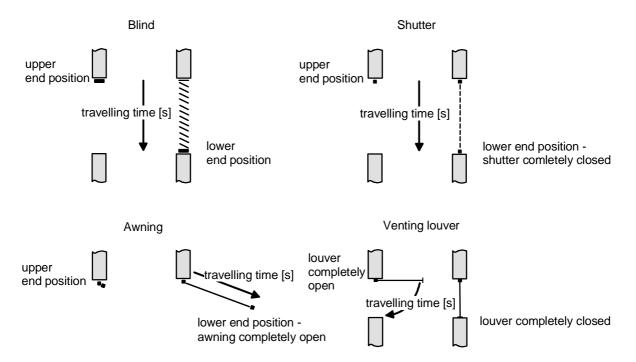
Fig. 9: Travelling time as a function of the type of movement
