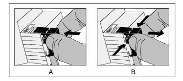
Fig. 5: Installing / removing the protective cap
