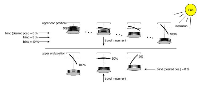
Fig. 14: Example of slat positioning with the blind in upper end position (typical of slat type 1)
