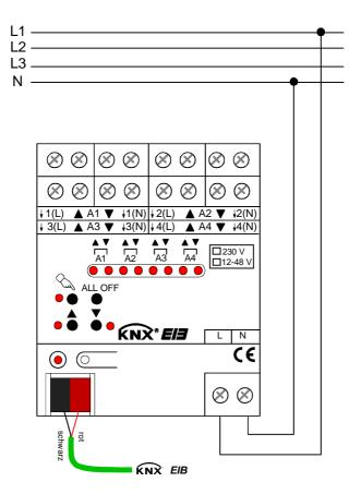
Fig. 1: Electrical connection of mains voltage
