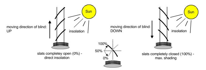
Fig. 10: type 1 - slatted blinds with oblique slat position in both travel directions
