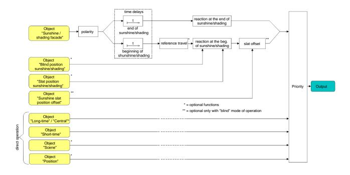
Fig. 19: Function diagram illustrating the simple sun protection
