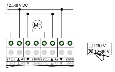
Fig. 4: Electrical connection for 12 ... 48 V drives
