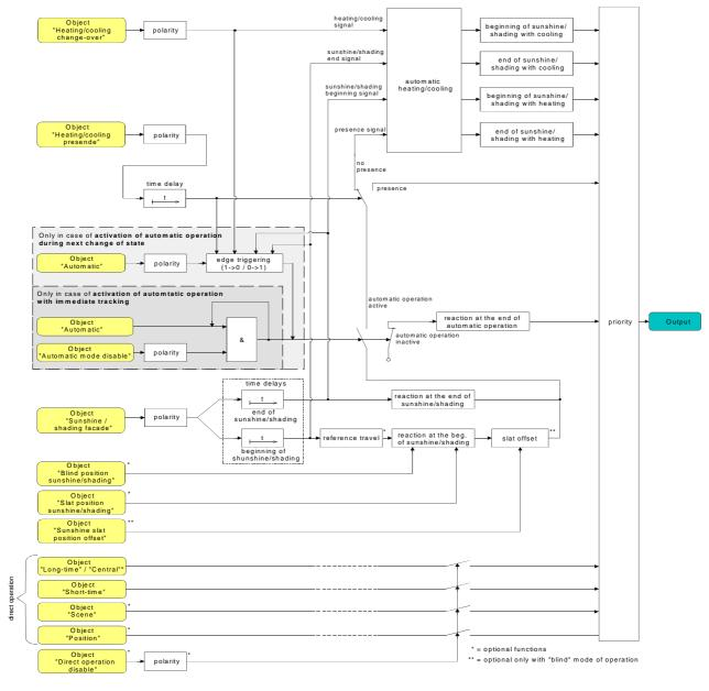
Fig. 29: Schematic diagram of automatic heating/cooling
