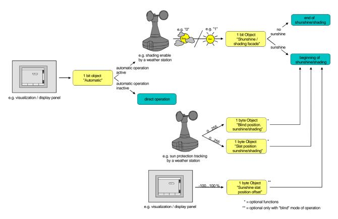
Fig. 20: Schematic diagram illustrating the enlarged sun protection configuration (for reasons of simplicity without disabling functions)
