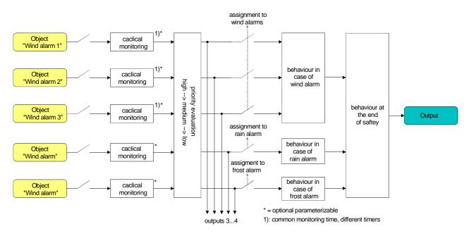
Fig. 16: Function diagram of channel-oriented safety functions
