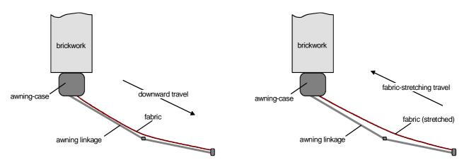
Fig. 30: Fabric-stretching in an awning
