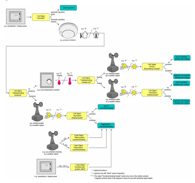
Fig. 28: Schematic diagram of the automatic heating/cooling system (for reasons of simplicity shown without disabling functions of the automatic or direct operation)
