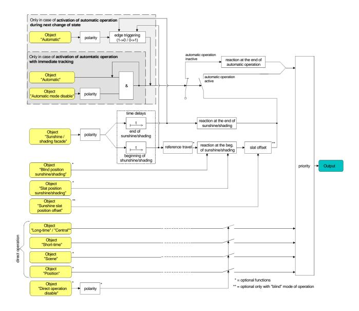
Fig. 21: Functional diagram illustrating the enlarged sun protection
