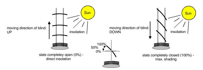
Fig. 11: Type 2 - slatted blinds with oblique and horizontal slat position
