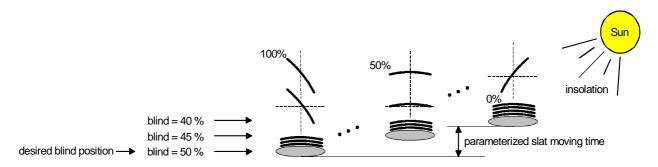
Fig. 13: Example of slat positioning affecting the position of the blind (typical of slat type 1; analogous reaction for type 2)
