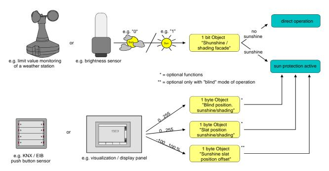
Fig. 18: Schematic diagram illustrating the simple sun protection configuration
