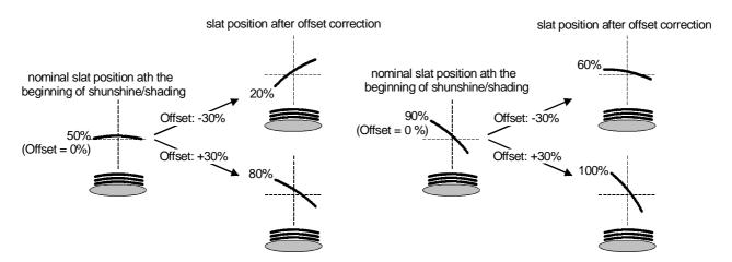
Fig. 22: Functional principle of slat offset (example showing slat type 1 / slat type 2 identical)
