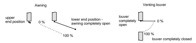
Fig. 12: Positions defined as a function of the type of movement
