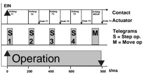
If the button is held after all step commands have been sent a continuous command (move) is sent to the bus in accordance with the set time (factor x base) that controls the actuators into the continuous mode.
