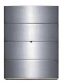
The B.IQ light scene push button comfort transmits telegrams to the instabus EIB when the button is activitated, which in turn triggers appropriate functions if actuators exist. Depending on the application that is loaded, you can save and re-use up to 8 background light scenes or telegram sequences with a maximum of 8 outputs.
