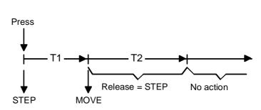
Pressing a key will transmit a step command and time T1 is started ("*time between step and move operation*") No other telegram will be transmitted, if the key is released within T1. This step serves to stop a continuous run in progress.
