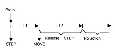
Pressing a rocker's key will transmit a step command and time T1 is started (*"time between step and move operation"*) No other telegram is transmitted, if the key is released within T1. This step serves to stop a continuous run in progress.
