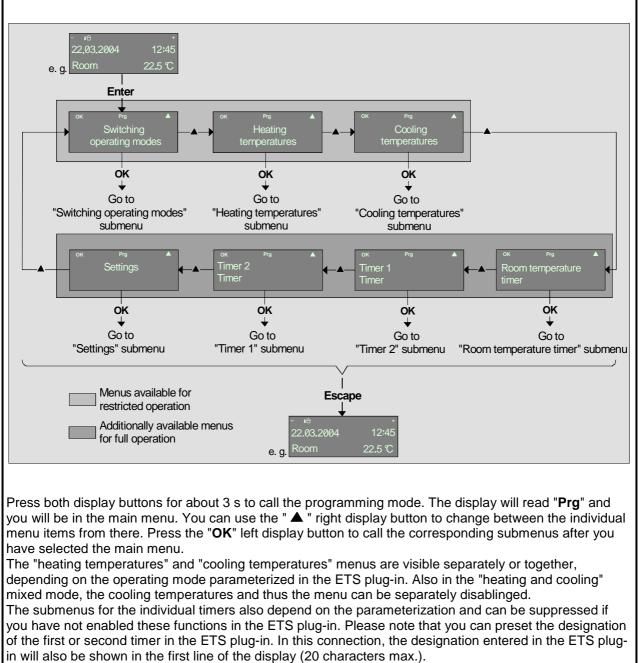
If you press any button of the push button (except the display buttons), or if you do not operate any button for about 20 s you will return to normal operation.
