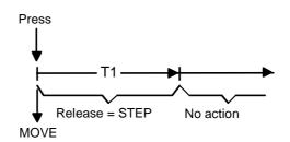
Pressing a key will transmit a Move command and time T1 is started ("Lamella adjustment time"). If the key is released again within T1, the push button will transmit a step-telegram. This function is used to adjust the Lamellas. T1 should correspond to the time required for a 180° rotation.
