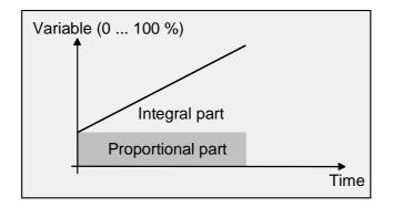
An additional heating or cooling stage as PI control works in the same way as the PI control of the basic stage, with the exception that the set value will shift, taking account of the parameterized step width.
