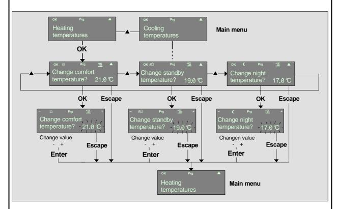
Once a setpoint has been set and the input has been confirmed by an **Enter** command, the operating mode associated with the adjusted setpoint will be accepted as the active mode. This, however, is only the case if <u>no</u> higher-priority mode (e.g. window contact / presence detector) is activated or if the KONNEX forced object is <u>not</u> activated!
