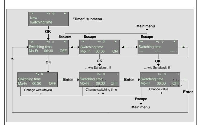
You can send switching commands (ON, OFF), value commands (0...255 / 0...100 %) or scene recall commands (1...8) to the bus and edit them from the programming menu. The data format (switching, value, scene) of the command to be transmitted is parameterized in the ETS plug-in and cannot be changed locally. Depending on the selection made in the ETS plug-in, the value range and the representation of the command are adapted in the programming menu.
