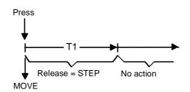
Pressing a rocker's key will transmit a Move command and time T1 is started ("*Lamella adjustment time*") If the key is released again within T1, the push button will transmit a step-telegram. This function is used to adjust the Lamellas. T1 should correspond to the time required for a 180° rotation.
