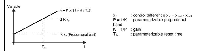
PI control algorithm: Actuating variable  $y = K x_d [1 + (t / T_N)];$  By deactivating the reset-time (setting = "0"):
