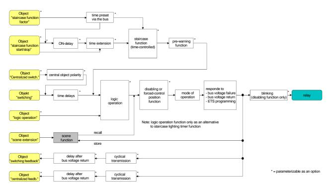
Fig. 15: Functional diagram of the scene function
