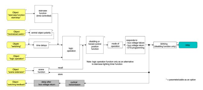
Fig. 7: Functional feedback diagram
