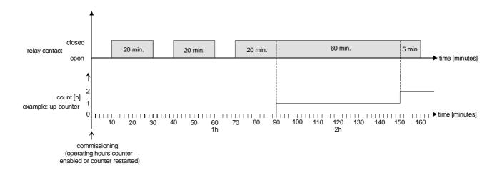
Fig. 16: Functional principle of the operating hours counter
