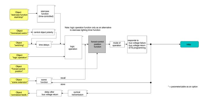
Fig. 18: Functional diagram of the forced-control position function
