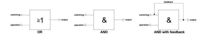
Fig. 20: Gating operations of the logic function
