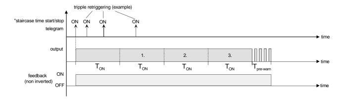
Fig. 14: Time extension for staircase lighting function
