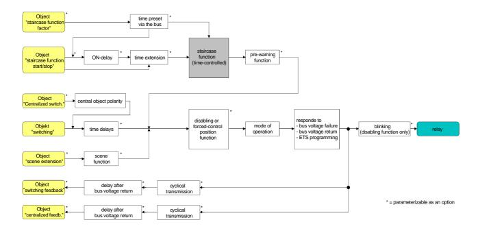
Fig. 10: Functional diagram of the staircase function
