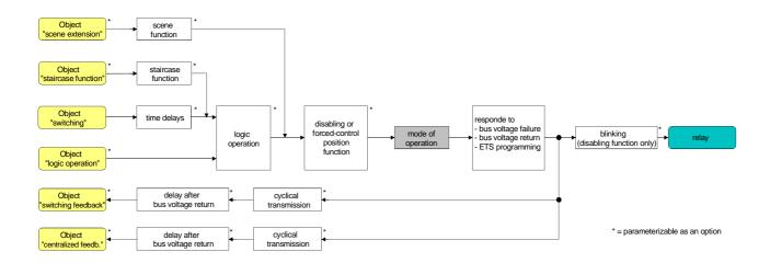
Fig. 6: Functional diagram "Mode of operation"
