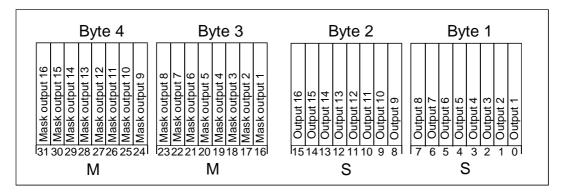
Fig. 5: Structure of the centralized feedback object
