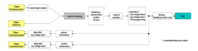
Fig. 8: Functional diagram of cyclical monitoring function
