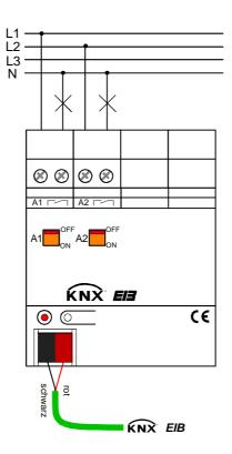
Fig. 1: Electrical connection
