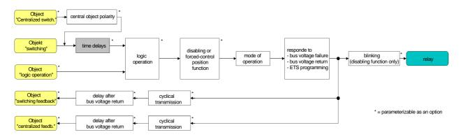
Fig. 9: Functional diagram of the time delays
