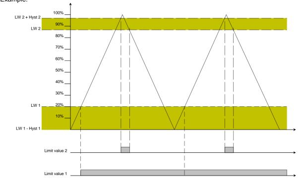
The limit values and the hysteresis characteristics are specified as a percentage of the full measuring range. When setting the limit values and the pertaining hysteresis, a safety margin of about 1% from the minimum value (0%) and from the maximum value (100%) should be observed. Or else the signals cannot underrun or exceed the respective thresholds. In this case, the limit-value object can transmit at maximum one telegram as shown for limit value 1.
