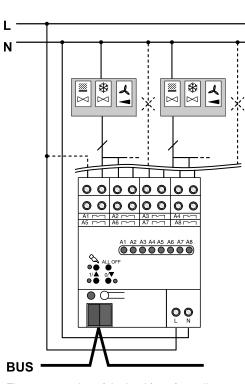
Fig. 6: connection of the load for 2 fan coil outputs
