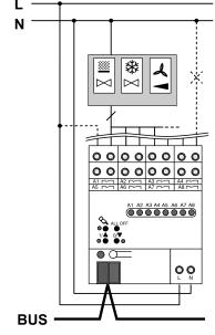
Fig. 3: connection of the load for 1 fan coil output
