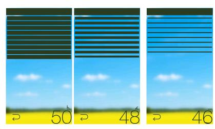
When the position of the lamellas change, the vertical position of the blind may change too according to received values.
